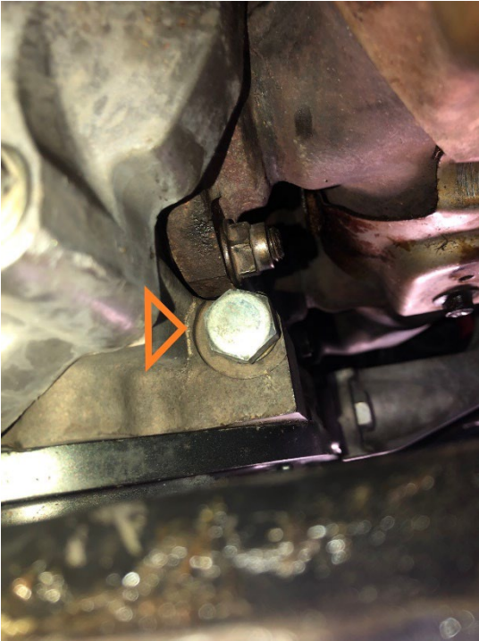
19.1.2 Differential Seal – The lower left bolt, and the adjacent bolt above on the left-hand side, as viewed from the rear of the differential.
